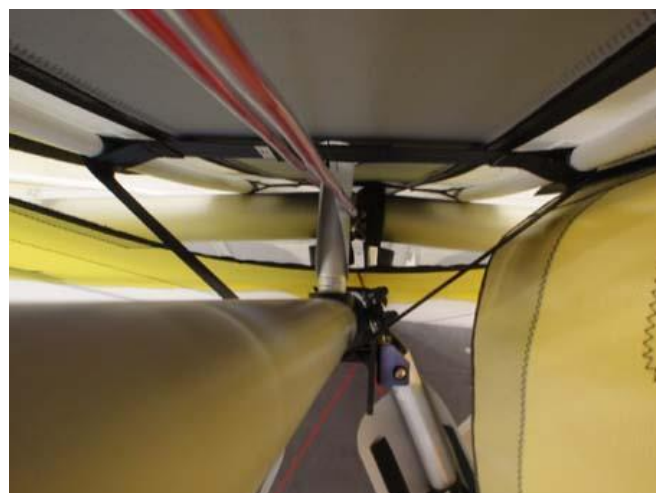
Figure 5-2 : Path of Tensioning Cables
